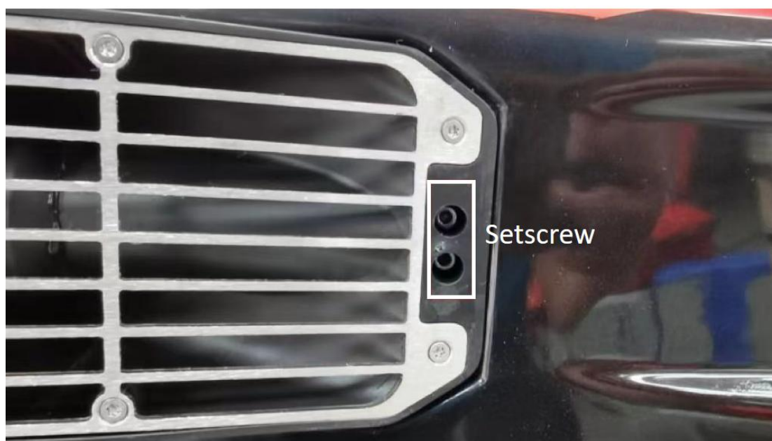
Figure 6-10 Securing the Propeller Screws
