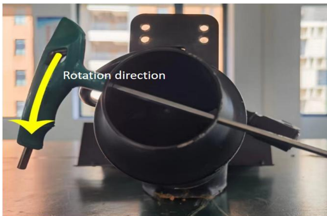
Figure 6-3 Direction of Rotation for Removing the Deflector
