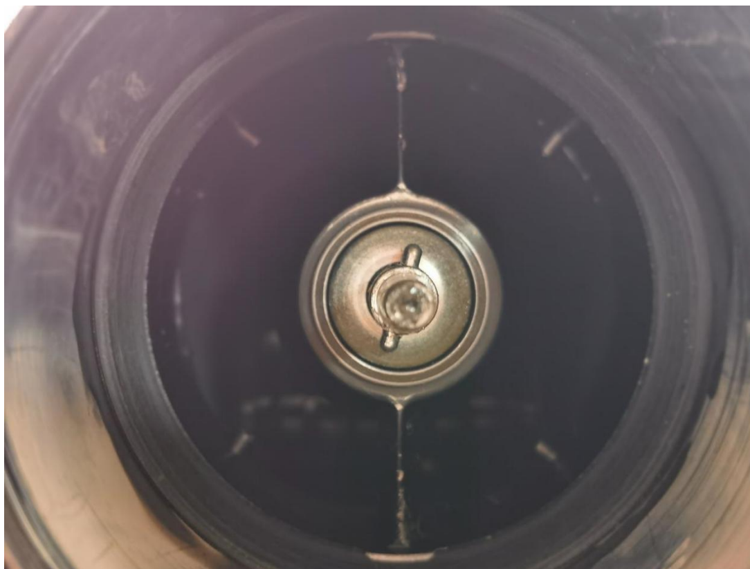
Figure 6-8 Securing the Propeller Blade Shaft
