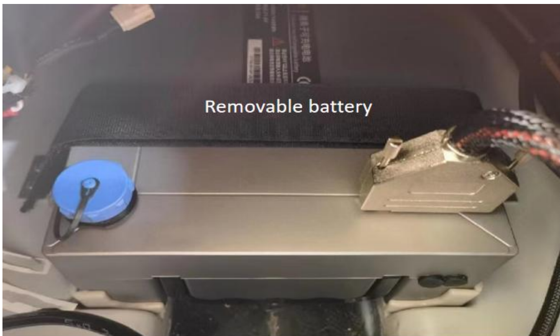
Figure 1-9 SinoGNSS SV600 Hull Battery Installation
